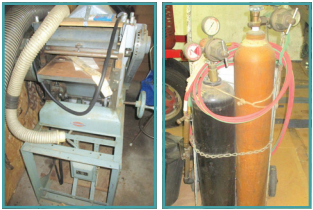
Craftsman industrial surface planer Acetylene tank & torch set
