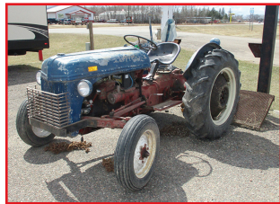
Ford 8N tractor with back blade & rear PTO
